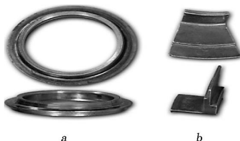
Fig. 9. Complicated profiled products obtained by rolling with a cylindrical roll: a —flange with a collar; b —element of the body of the electrovacuum device.
